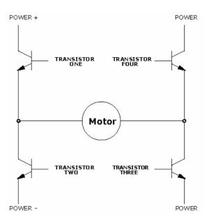
There are Hbridges in a chip such as the one described here: <a href="http://profmason.com/?p=243">http://profmason.com/?p=243</a>
